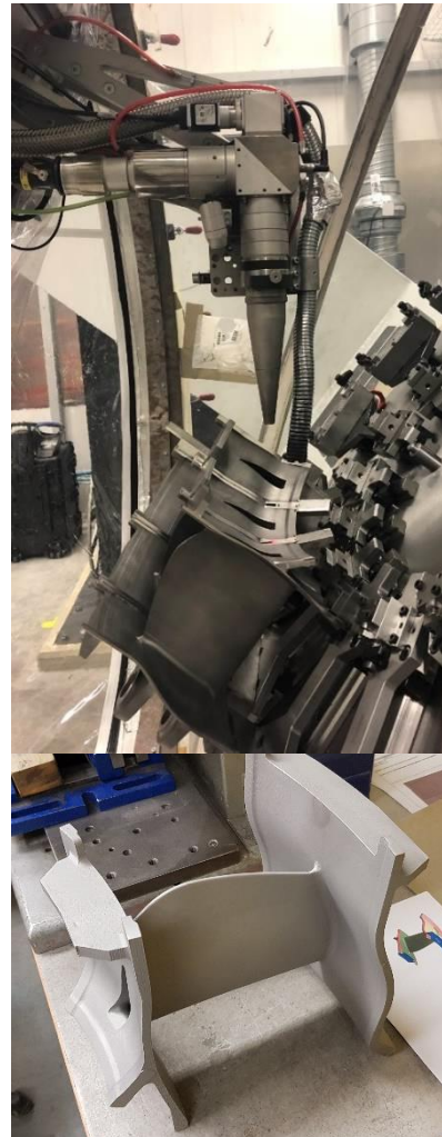
Figure 3. The final demonstrator will probably consist of two super alloy sectors (as above) welded together. Size is typically 25 cm in all dimensions.
