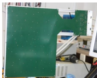
Figure 2: Example of microphone array containing 64 sensors.
