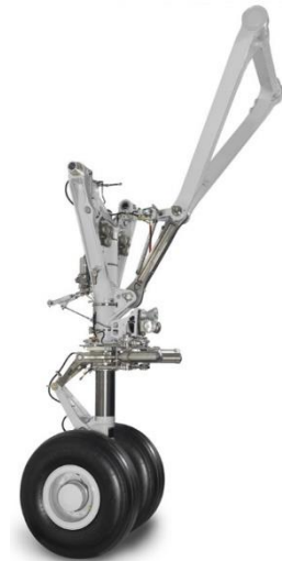
Figure 1: A350 Nose Landing Gear with Main Fitting and Sliding Tube made of 300M UHS © Liebherr Aerospace
