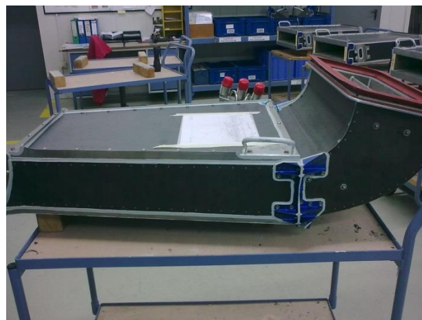
Figure 4 Example of Air intake ducting
