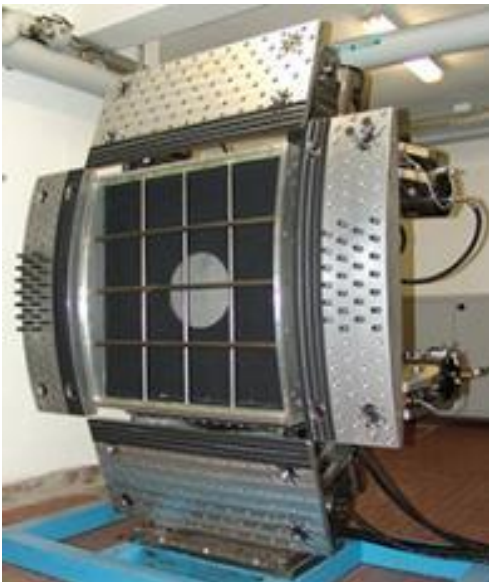
Figure 3: Example of fuselage panel test (courtesy AESDO/POLITO)
