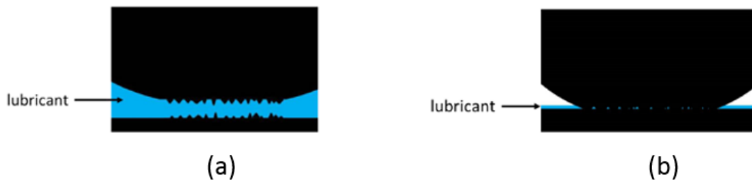
Pictorial representation of solid material contact with full lubrication (a) and boundary/starved lubrication (b). Condition (b) may lead to material scoring/damage.
