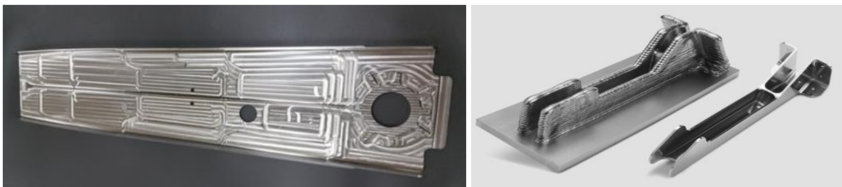
Figure 2. (LEFT) Study case for Airbus upper rear spar component in Ti6Al4V printed using Sciaky W-DED EBAM [1]. (RIGHT) First FAA-certified Ti6Al4V Structural component galley bracket for Boeing 787 Dreamliner printed using Norsk Titanium W-DED WAAM [2].
